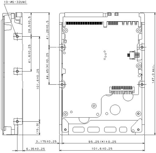
The value marked with (\*) indicates the dimension between mounting holes on the bottom face.
